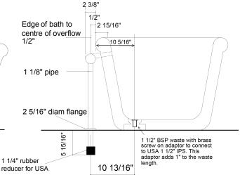
Waste: 1 1/2" BSP // 1 1/2" IPS; Overflow: 28mm / 1 1/4" rubber reducer.
