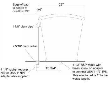
Waste: 1 1/2" BSP // 1 1/2" IPS; Overflow: 28mm / 1 1/4" rubber reducer.
