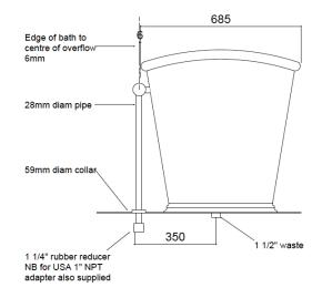
Waste: 1 1/2" BSP; Overflow: 28mm / 1 1/4" rubber reducer. We only supply fittings above the floor. We do not supply the trap; the trap needs to go beneath the floor. Dimensions are given in mm; they are a guide only and may vary from bath to bath.
