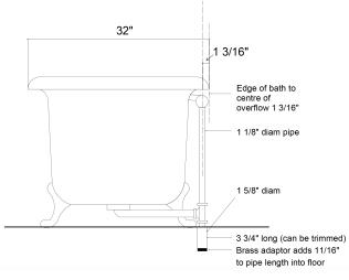
The outlet pipe can be used horizontally by turning the 'T' and can be supplied with an extra pipe and elbow if wishing to go into the floor further behind the bath if specified.
