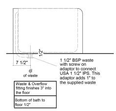
Combined waste and overflow 1 1/2" BSP, supplied with adaptor to connect to USA 1 1/2" IPS. We only supply fittings above the floor. We do not supply the trap; the trap needs to go beneath the floor. Dimensions are given in inches, they are a guide and vary from bath to bath.
