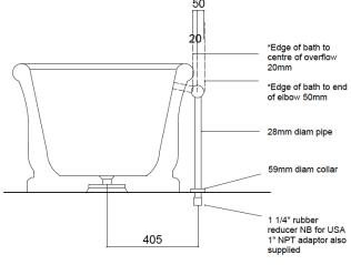
Waste: 1 1/2" BSP; Overflow: 28mm / 1 1/4" rubber reducer.
