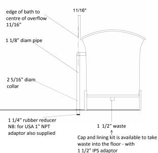
Waste:  $1 \frac{1}{2}$  BSP; Overflow: 28mm into 42mm waste pipe - outlet is UK  $1 \frac{1}{2}$  BSP - USA  $1 \frac{1}{2}$  IPS. We only supply fittings above the floor. We do not supply the trap; the trap needs to go beneath the floor. Dimensions are given in inches; they are a guide only and may vary from bath to bath.
