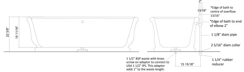
Waste: 1 1/2" BSP; Overflow: 28mm / 1 1/4" rubber reducer.
